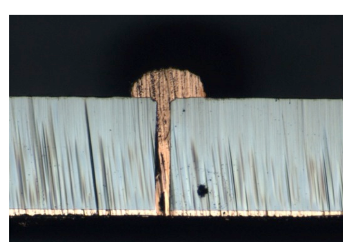
Coloured SEM image of copper through-wafer vias
