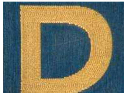
<5% Spot Overlap low resolution “scallop” edge
