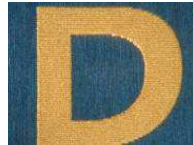
>60% Spot Overlap high resolution smooth line edge
