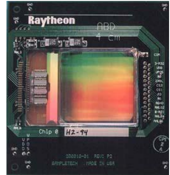
Phased array deflectors Single line scanning Scanning angles > 20^\circ Scanning speed > 500 m/s for EO-devices
