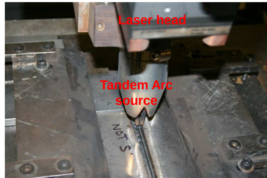
Tandem arc – laser hybrid set-up
