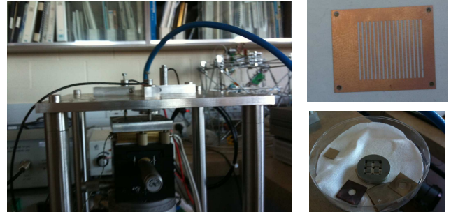
Fig.3: Rig (left) and LCP mask design (top right) and nickel masks (bottom right)
