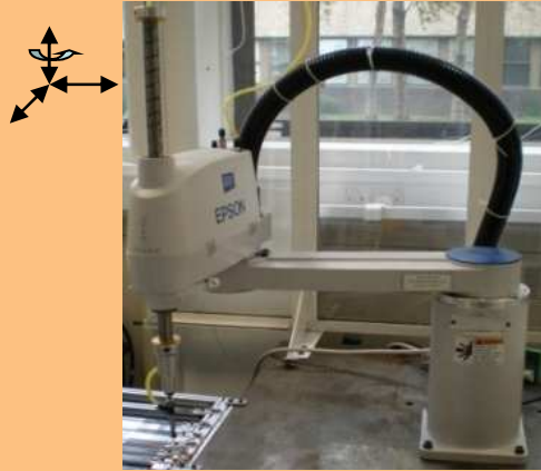
SCARA (serial) manipulator
